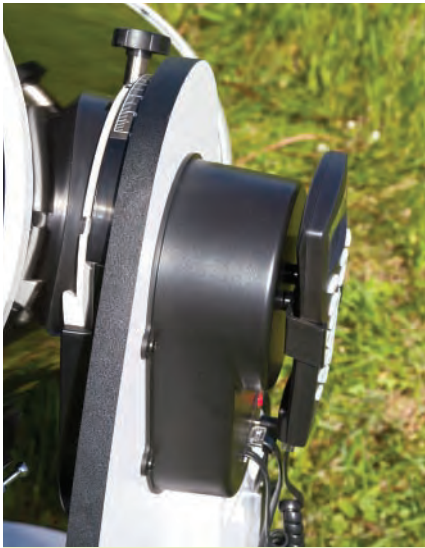
GETTING A BEARING The tube's trunions slide down into channels on the mount's side bearings, making for quick assembly in the field.
