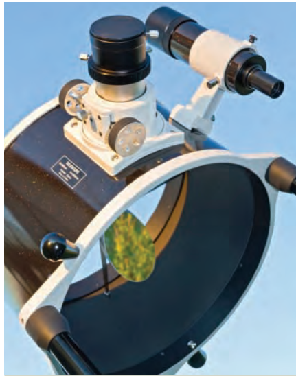
FITTED OUT The excellent 8x50 finder-scope is easily removable. The single-speed focuser is a smooth, precise Crayford design.
