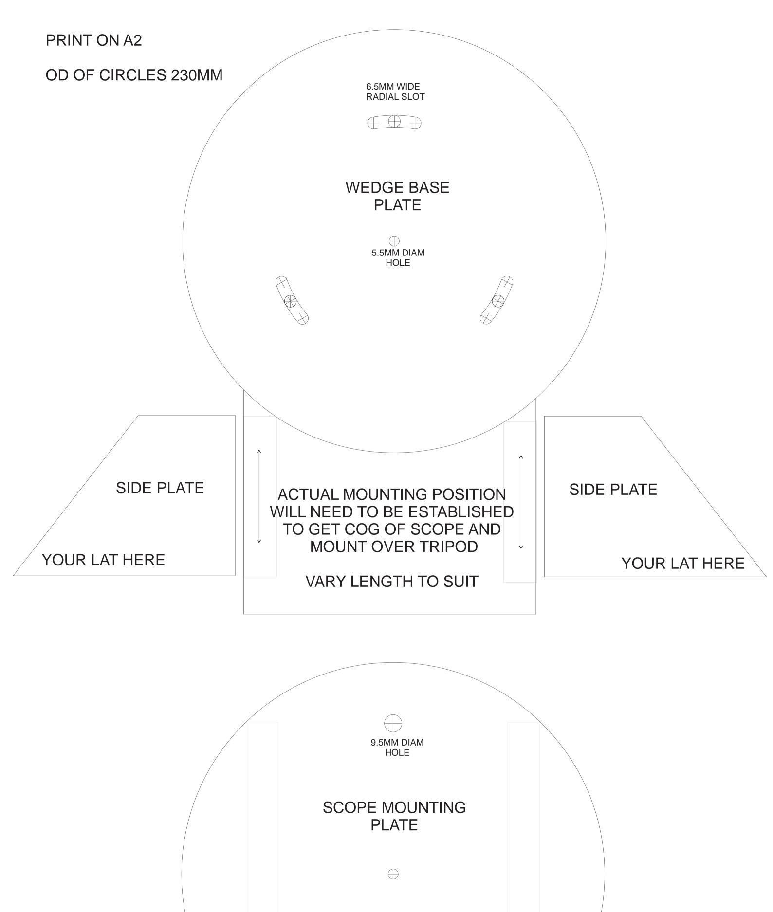
ADJUST DETAIL TO SUIT BOLTS WASHERS THAT ARE ACTUALLY USED PROB 3/8 Whitworth
