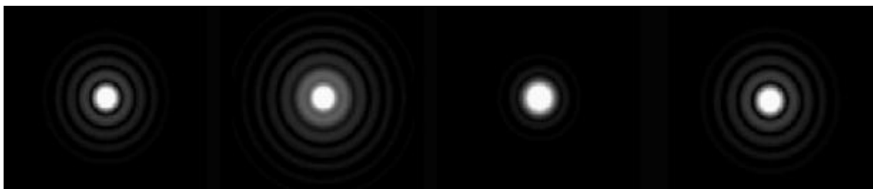
From left to right: perfect unobstructed image, image with severe rolled edge, apodized severe rolled edge, image as it would be if we merely stopped down below the edge difficulty.
