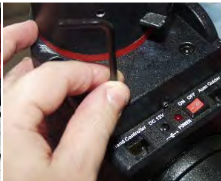
Replace the cap head bolts (normally silver coloured) with just enough pressure to hold the worm carrier in place. Make sure the carrier is lined up with the mount.
