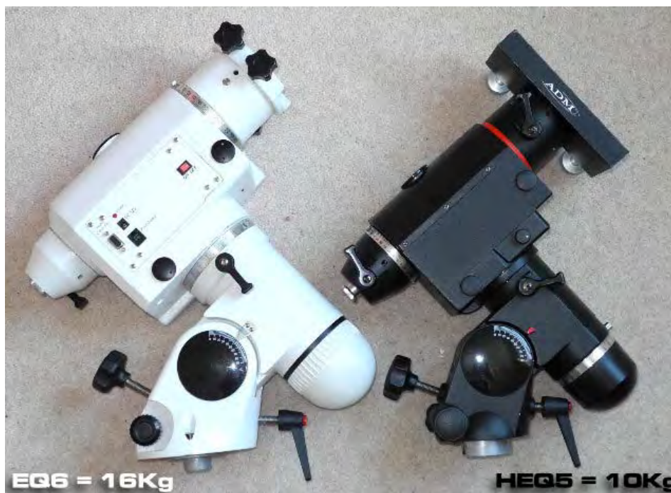
An EQ6 / NEQ6 Pro alongside a standard HEQ5. Pro versions with GoTo are mostly white while the non-GoTo versions are most usually black. Weights for the mount head are given.
