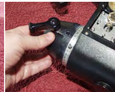
Replace the counterweight collar. Tighten this down using only hand pressure. Tighten it as far as it will go and then back off until the counter-weight lock lever is in line with the Declination lock lever.
