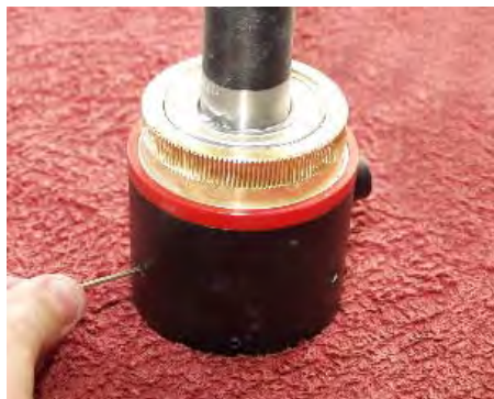
Tighten down the 3 deep set screws on the Declination barrel.
