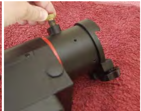
Remove the brass declination lock bolt. You may need to use a small spanner or pliers to loosen it.
