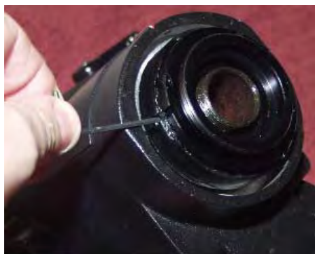
Loosen the three lock screws set around the large circular aluminium nut.
