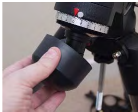
Replace the polarscope cover. The polarscope will require recalibrating. See my polar alignment guide HERE
