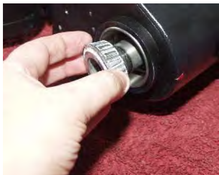
Replace the tapered bearing at the bottom of the main housing after lubricating it with lithium grease. Note If this wont push all the way in dont worry. As long as there is some thread showing on the Dec shaft for the counterweight collar.
