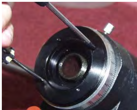
Now remove the polarscope mounting plate by unscrewing it. You can use either some snipe nosed pliers to locate into the holes OR a pair of small/medium Phillips screw drivers or similar OR a pair of small Allen keys.
