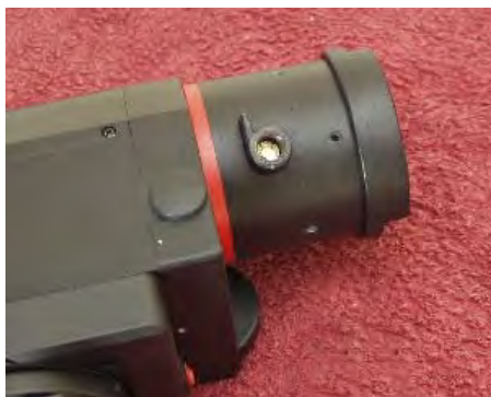
Remove the small 'button' if this didn't come out with the lock bolt. If you cant get this out don't worry it can be removed at a later stage.
