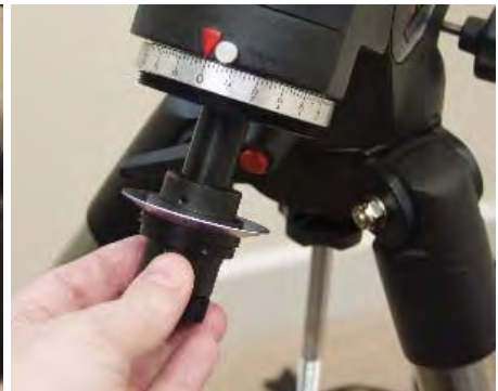
Once loosened simply unscrew the polar scope and place it somewhere safe.
