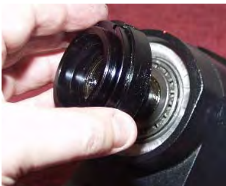
Unscrew and remove the circular nut. You may need a wrench to do this - if so be careful of the polar-scope mounting plate threads. Alternately use a pair of flat bladed screwdrivers or similar to apply even pressure using the slots in the nut - do this with care . Once removed observe the tapered bearing. It may come out at this point - if not it can be removed easily after the following step.
