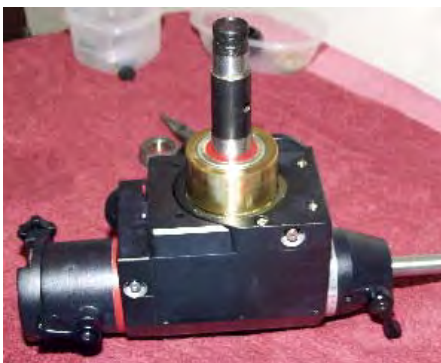
Unscrew and remove the circular nut. You may need a wrench to do this - if so be careful of the polar-scope mounting plate threads. Alternately use a pair of flat bladed screwdrivers or similar to apply even pressure using the slots in the nut - do this with care . Once removed observe the tapered bearing. It may come out at this point - if not it can be removed easily after the following step.
