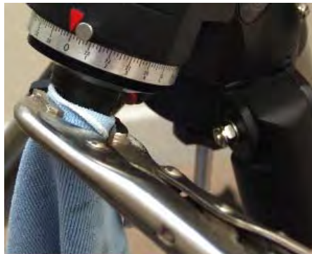
Remove the polar scope. You may need to grip it with a wrench - if so wrap a cloth around the polar scope to protect it. Alternately use some masking tape to protect the scope.
