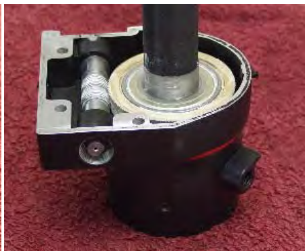
Replace the worm carrier onto the Declination shaft. Replace the clear washer on top of the brass gear. Its almost invisible in the picture above.
