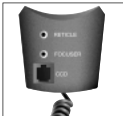
Fig. 16: #909 Accessory Port Module (APM).
