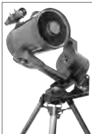
Fig. 24: Tripod set in Polar configuration with an optional wedge.
