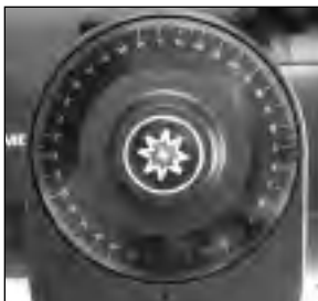
Figure 28: Section of Declination Setting Circle.
