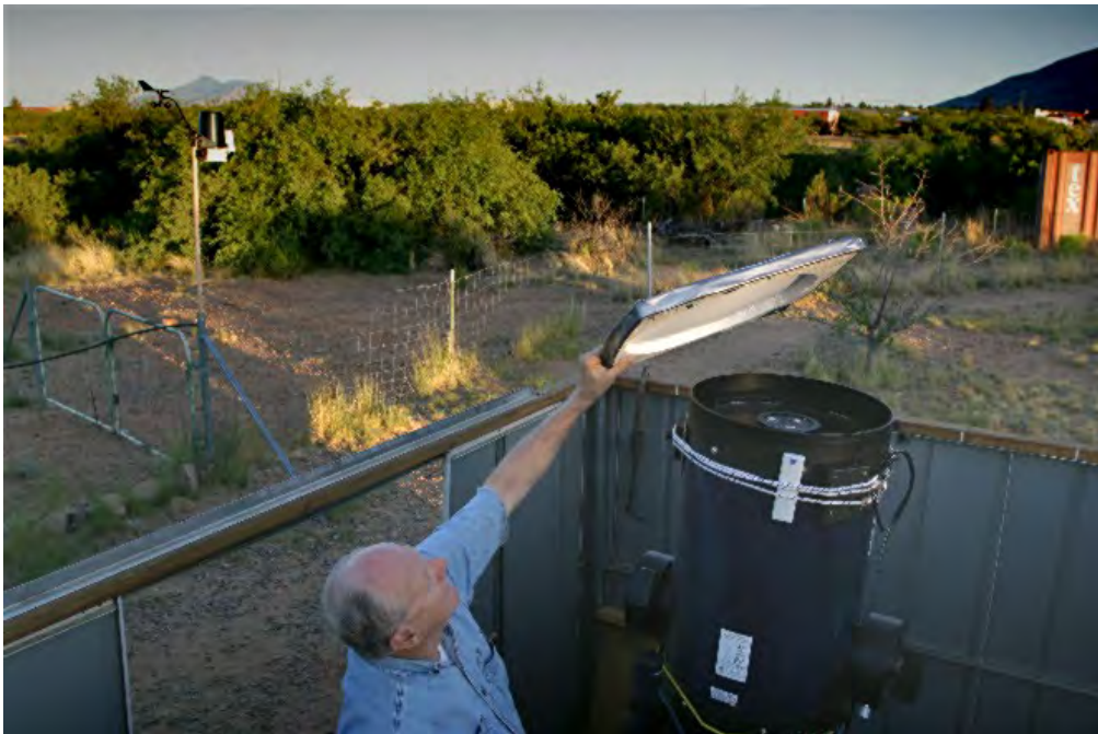
Figure 5.01. Double T-shirt diffuser is being placed on top of the telescope aperture for obtaining flat fields. (The Davis Weather Station is in the background.)
