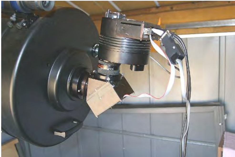
Figure 2.02. My favorite configuration: AO-7, focal reducer, CFW/CCD (SBIG ST-8XE). The telescope is a Meade LX200GPS 14-inch aperture, f/10 (without a focal reduce.).
