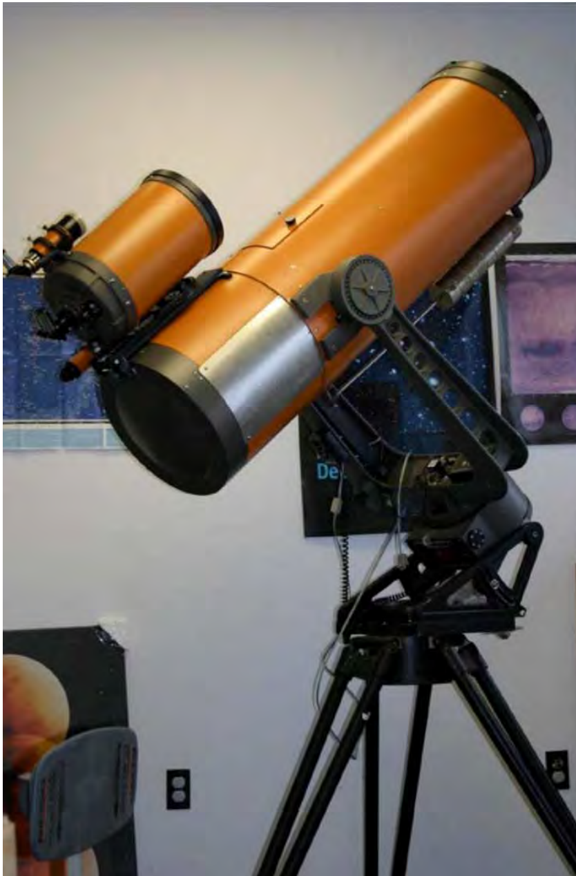
Fig. 48-36 This beautiful 14-inch Schmidt camera is equipped with an orange-tube C8 guidescope, mounted to the camera with the LARGE-SIZE Celestron tangent coupler. (Courtesy of Peter Fassler)
