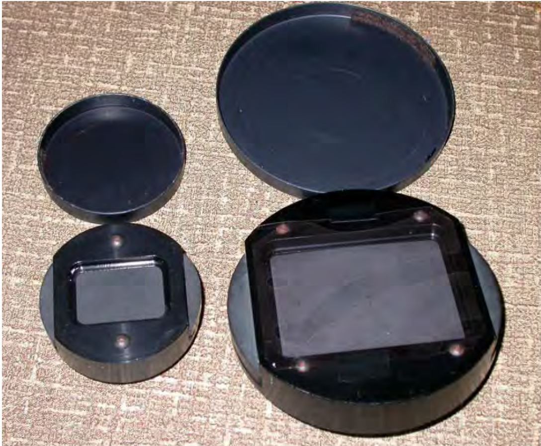
Fig. 48-38 35mm and 120 filmholders for the 14-inch Schmidt camera. The 120 holder has a thin Wratten filter taped over it, barely visible in this photo.
