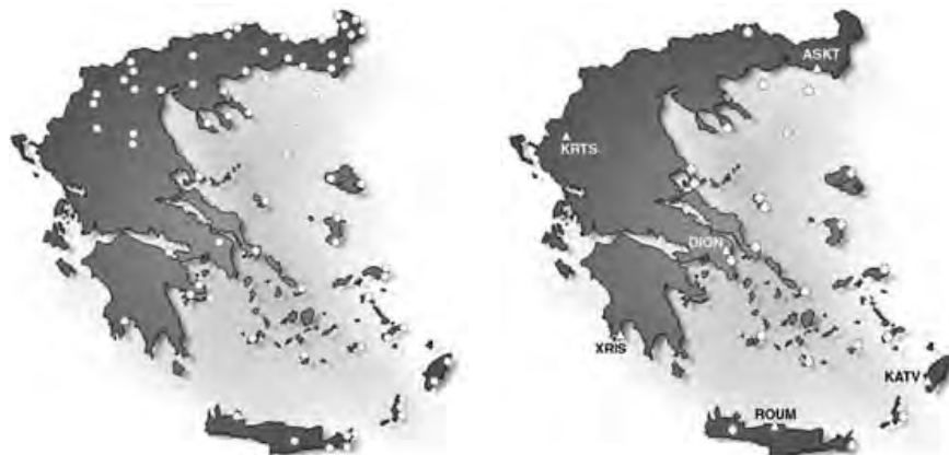
Figure 2 - Parts of the AEGEANET network consisting of 66 pillars of the national geodetic network (left) and 4 SLR pads and 22 previously established GPS markers (right).
