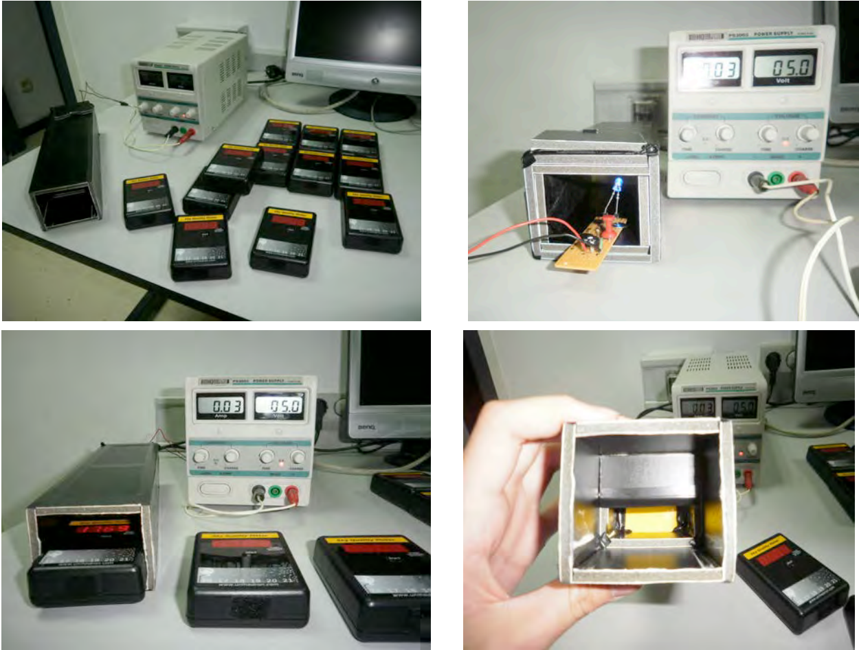
Figure 1-4. : Laboratory experimental setup consisting in a stable power supply and a black box where the blue LED and the yellow filter are placed.
