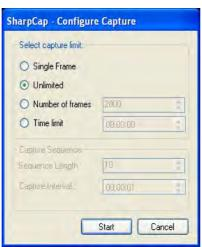
12. Set your drift path and once the planet appears on the screen, hit **start**. MAKE SURE THE PLANET IS 100% VISIBLE, EXCEPT WHEN IT IS ENTERING AND EXITING THE SCREEN. Once the planet leaves the screen on the right hand side, click **stop capture**. Repeat this process and aim to capture at least 15 good videos. Don't touch the telescope whilst you are capturing. When this is done, bring all the kit back inside.
