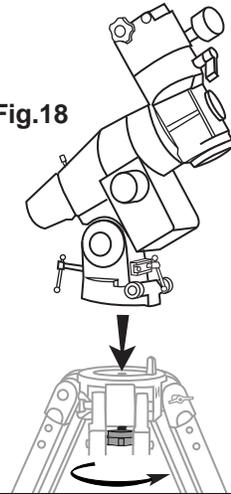
Note: Loosen the azimuthal adjustment knobs if mount does not fit into tripod head completely. Retighten knobs to secure.
