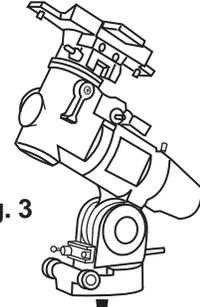
Note: Loosen the azimuthal adjustment knobs if mount does not fit into tripod head completely. Retighten knobs to secure.
