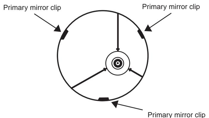
alternately loosen one and then compensate for the slack by tightening the other two. Stop when you see all three mirror clips (Fig.s4). Make sure that all three small alignment screws are tightened to secure the secondary mirror in place.
